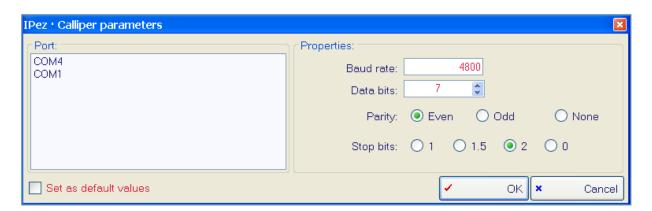
To know to which port the calliper is connected, go to "Control panel", then "System", followed by "Hardware", and "Device manager" within that window and, finally, into "Ports (COM & LPT)".
